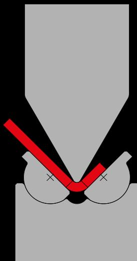
Sheet metal is always supported during bending
